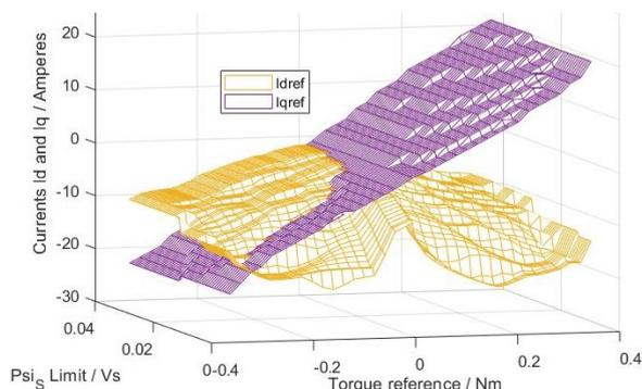
Figure 1: Recommended direct and quadrature currents depending on the operating conditions.
