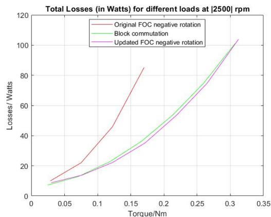
Figure 2: Losses as a function of load at 2500 RPM. FOC (red), BC (green), updated FOC (purple).
